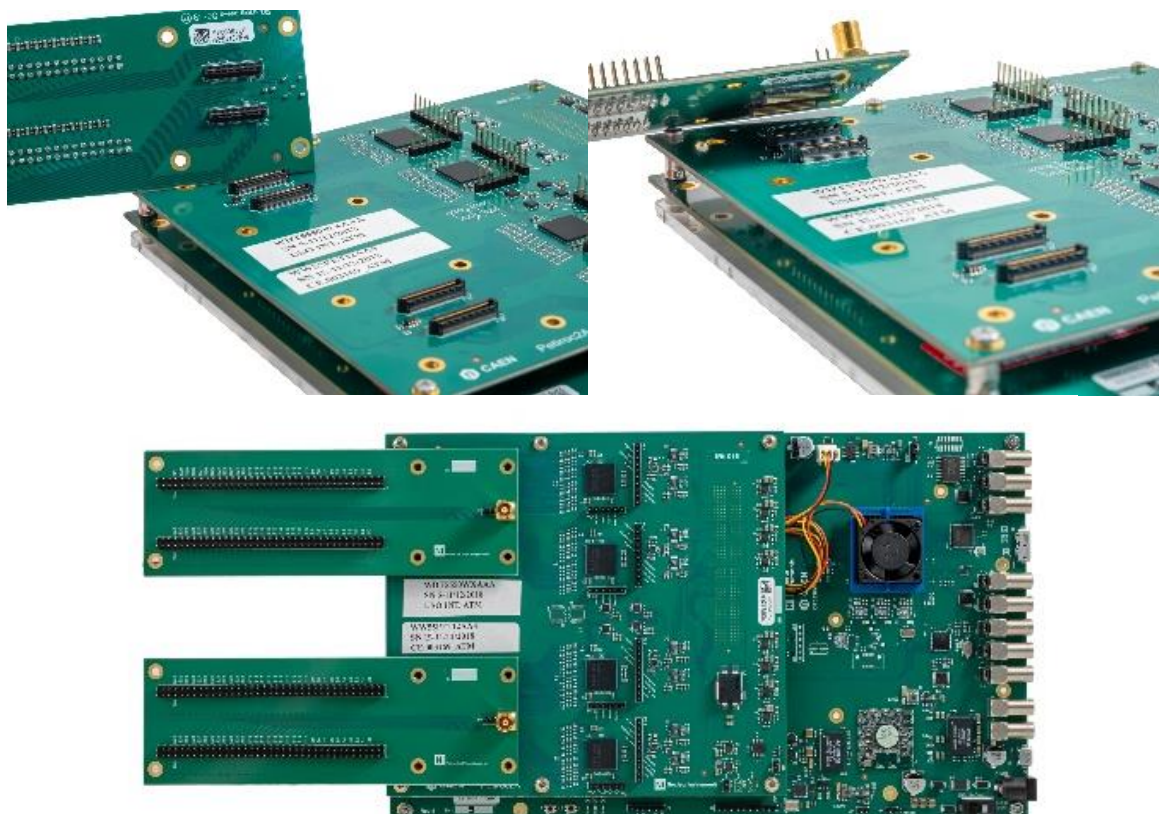
Figure 10.7: Top: how to plug the pitch adapter on the board's SiPM connector. The connectors are pressure-pluggable. Bottom: general view of a DT5550W with A55PET4 piggyback and two pitch adapters plugged in. In this configuration, all 128 channels of the DT5550W board are exposed on the strip connectors.
