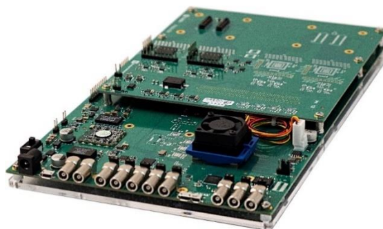
Figure 5.1: general view of the DT5550W system, where the piggyback is the upper board.
