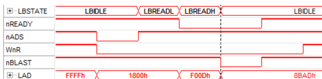
Fig. 12.4: Local bus signal at a read access (x8BADF00D is read from register x1800)
