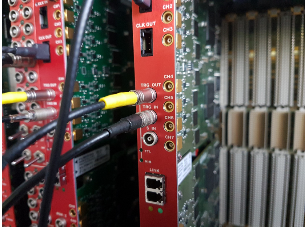
Fig. 4.3: The signal from the TRG OUT connector must be used to veto the global trigger
