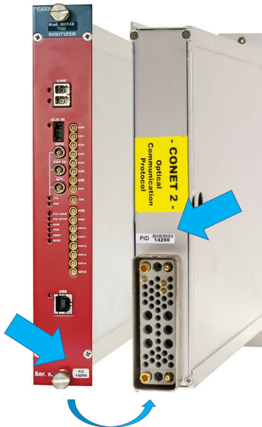
Fig. 5.1: PID location on N6742 (the number in the picture is purely indicative)
