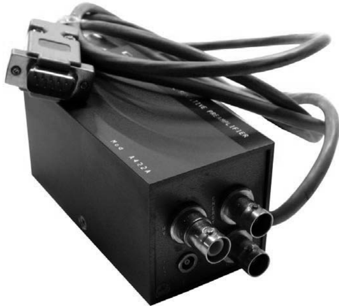
Fig. 1.1 – Mod. A422 A Charge Sensitive Preamplifier
