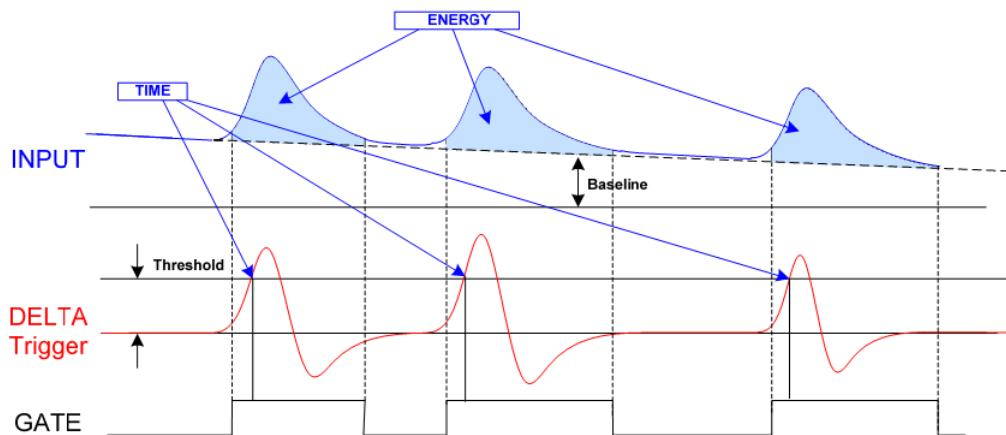
The delta signal recognizes the input pulses mitigating the influence of noise and baseline fluctuations, the trigger (identifying the arrival time) is generated as soon as this 'delta' is greater than a programmable digital threshold.
