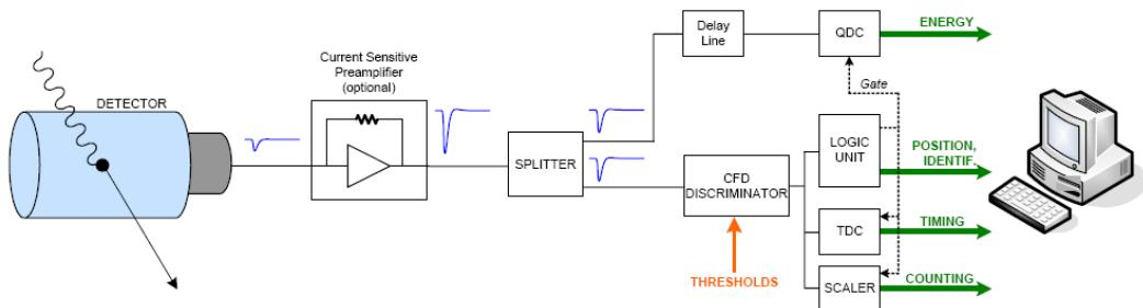
The following figure shows instead the block diagram of the digital QDC solution based on a waveform digitizer equipped with Digital Pulse Processing (DPP) firmware for Charge to Digital Conversion.
