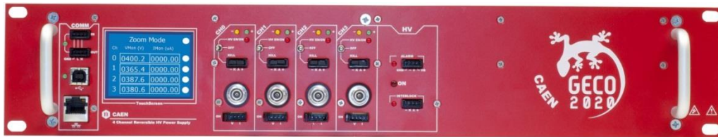
Fig. 3: R14xxET Front panel (4 channel)
