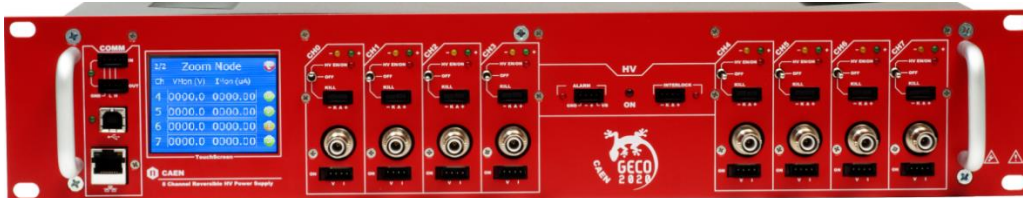
Fig. 4: R14xxET Front panel (8 channel)
