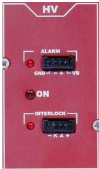
Fig. 12: HV Status control panel
