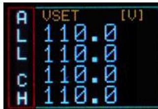
Push the TUNE ROTARY SWITCH: at this point the parameter is selected, its frame is shown in red and its name in blue (only one value common to all channels; pre-set value is picked from Channel 0); it is now possible to change the parameters value.
