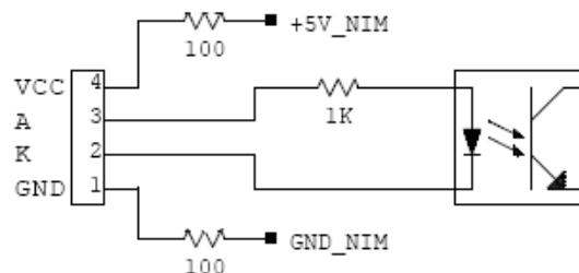
A schematic diagram of the Interlock input is shown in the figure above, where the diode is part of optocoupler stage.
