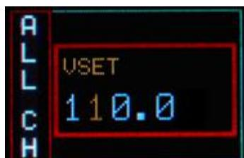
Turn the TUNE ROTARY SWITCH until the digit reaches the desired value
