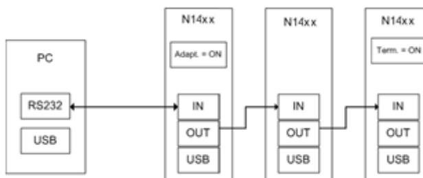
In order to control the module via RS232 it is necessary to use the module's COMM IN port (refer to p.8 for RS232 signals) and to follow adaptation instructions (see p.31).
