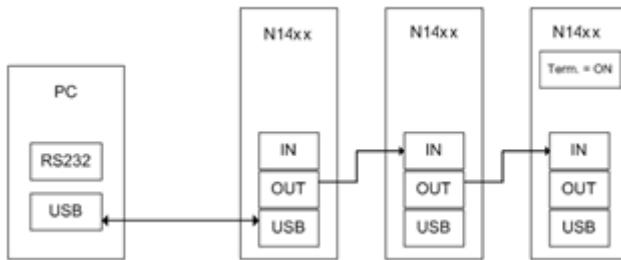
The module is provided with a USB2.0 compliant interface (see p.6). The N1410 can be programmed via PC by connecting the PC USB port with the N1410 USB B-type port; the featured controller, the FT232BM chip requires drivers freely available at [www.ftdichip.com](http://www.ftdichip.com) (Drivers section); the site also provides installation instructions for all OS's (Documents section)
