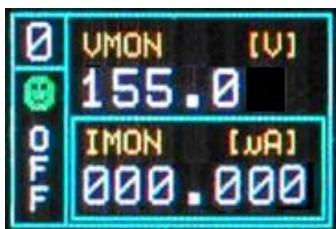
The KILL position of the HV\_EN/OFF/KILL 3 POS. SWITCH allows to turn off the module at the fastest available rate; the Display will show the following message in the left lower row:
