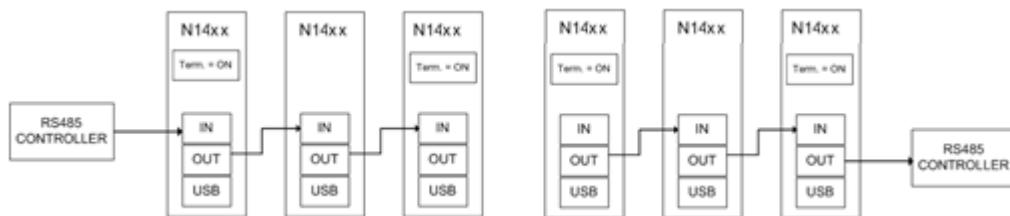
The COMM IN / OUT connectors implement a RS485 type LOCAL BUS which allows to build a 32 modules daisy chain. This can be achieved through the following steps:
