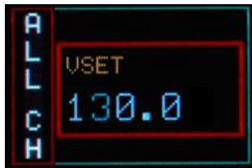
Once all the digits are set to the desired value, turn the TUNE ROTARY SWITCH until the parameter name returns blue. Push the TUNE ROTARY SWITCH to de-select the parameter, the frame returns to blue; when the parameter is not active, the parameter status of the four channels is shown.
