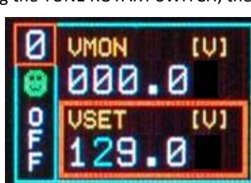
Once all the digits are set to the desired value, turn the TUNE ROTARY SWITCH until the parameter name returns blue
