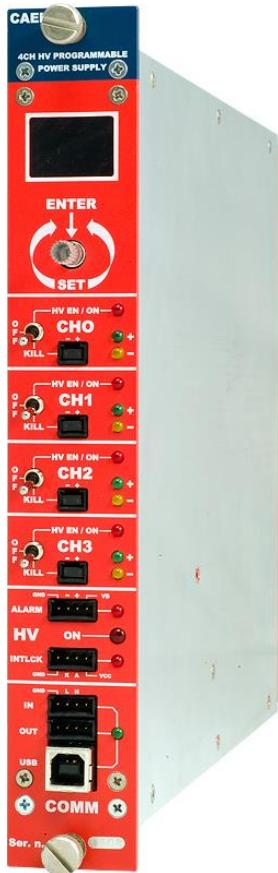
The Mod. N1410 provides 4 independent High Voltage channels in a single width NIM mechanics.
