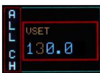
Confirm it by pushing the TUNE ROTARY SWITCH, the edited digit returns blue
