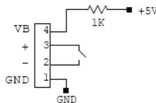
As an Alarm condition is detected (see p. 26 and 27) pins 2 and 3 (- and +) are closed; the contact can be used to switch an external device supplied by an external source, otherwise the VB and GND references can be used to provide a TTL compatible level on pin 2 and 3.
