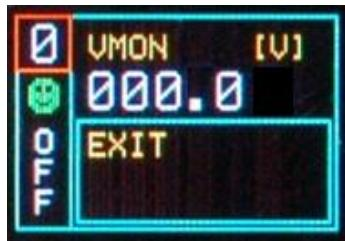
Now by turning the TUNE ROTARY SWITCH another channel number to be set can be selected.
