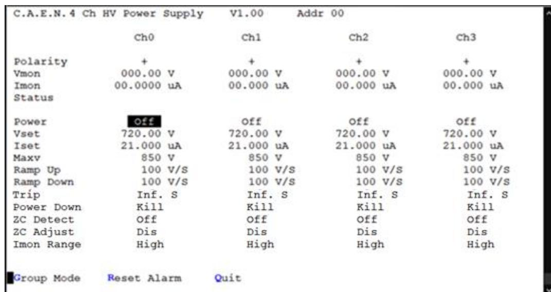
To change one parameter: point the parameter with the arrow keys (see figure below), and type the desired value, confirm by pressing <Enter>; Power, Power Down, ZC detect/adjust can be changed using the <Space> bar.
