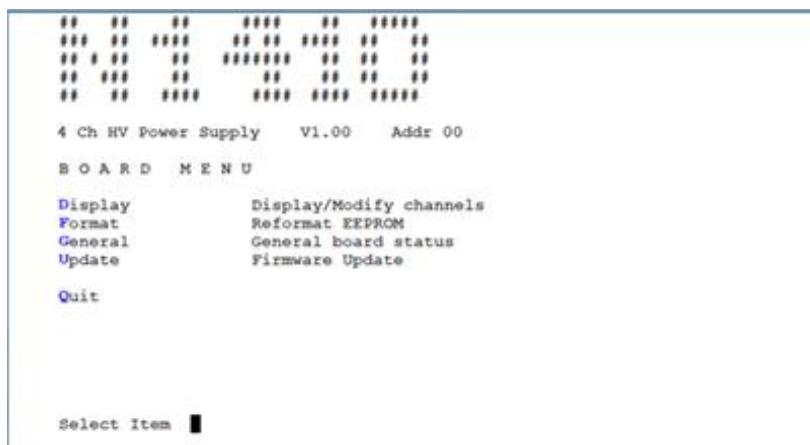
Type **D** to set/monitor channels parameters
