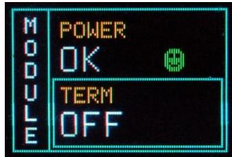
Push the TUNE ROTARY SWITCH in order to access MODULE parameters; the MODULE frame becomes red:
