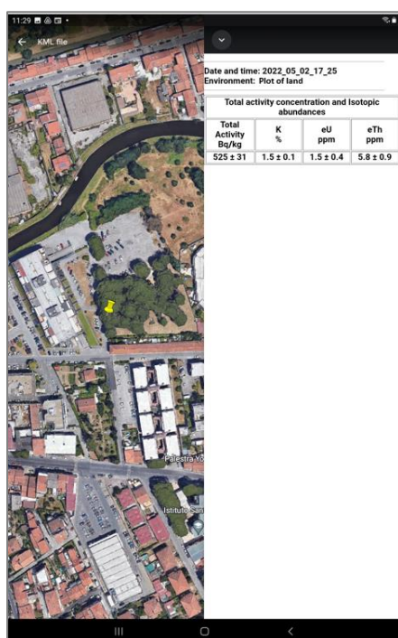
Fig. 4.7: Example of results of environmental radioactivity measurements visualized via Google Earth and obtained by GammaEDU in Viareggio (Tuscany - Italy).
