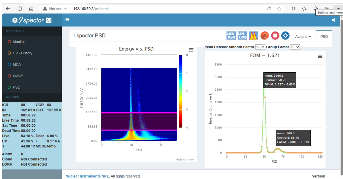
Figure 9.15: example of the PSD tab view. On the left it is possible to see the PSD vs. E scatter plot. On the right, it is possible to see the PSD vs. Integral counts for an interval of Energies that can be selected on the scatter plot with the magenta cursors.
