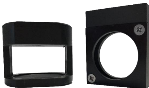
Fig. 5.5: Plastic holders allow horizontal and vertical source position
