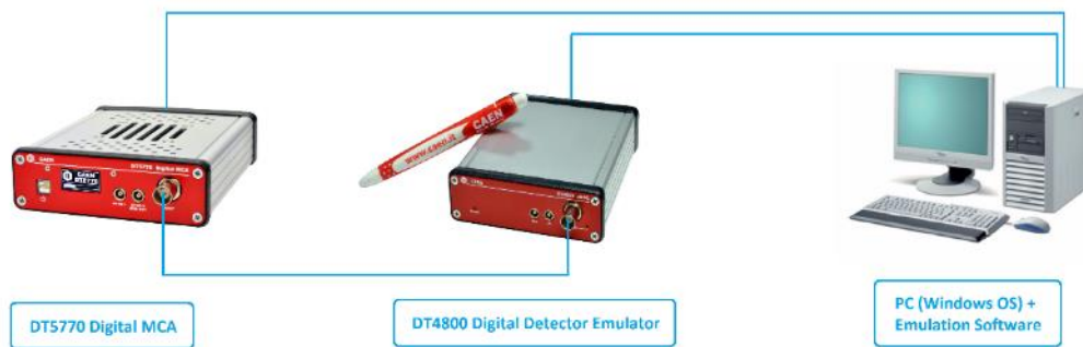
Figure 2.5: The hardware setup including the Digital Detector Emulator DT4800 and the Digital MCA DT5770.
