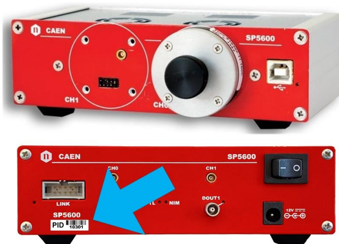
Fig. 3.2: SP5600 - Power Supply and Amplification Unit: PID position is located on the back panel of the module hosting the power input. Same location is adopted for DT5720A - Desktop Digitizer also.
