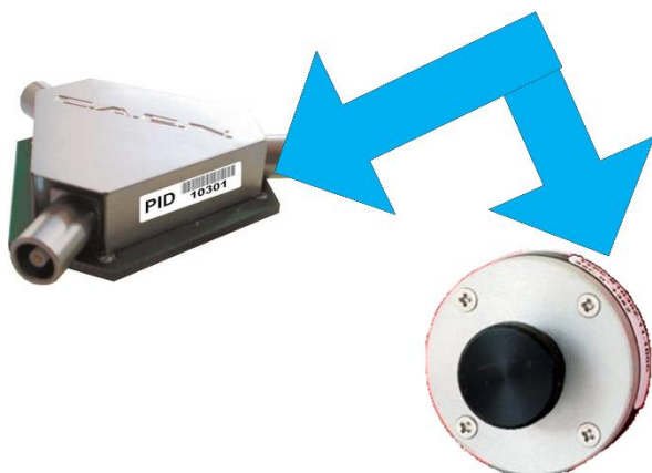
Fig. 3.3: PID position: on the metal shield for the A315 . Splitter or around the holder for the SP5650C - Sensor Holder with SiPM.
