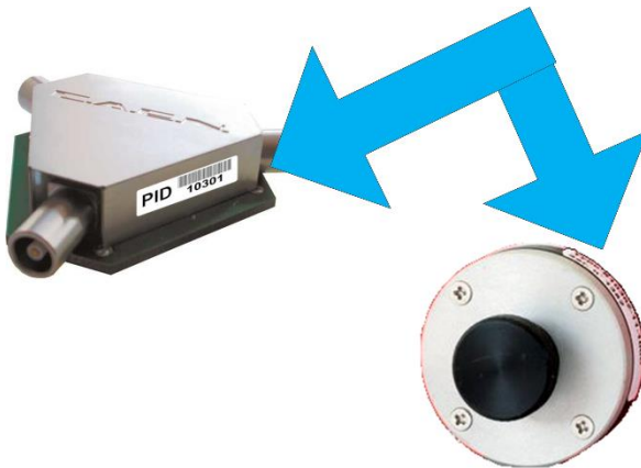
Fig. 3.4: PID position: on the metal shield for the A315 . Splitter or around the holder for the SP5650C - Sensor Holder with SiPM.
