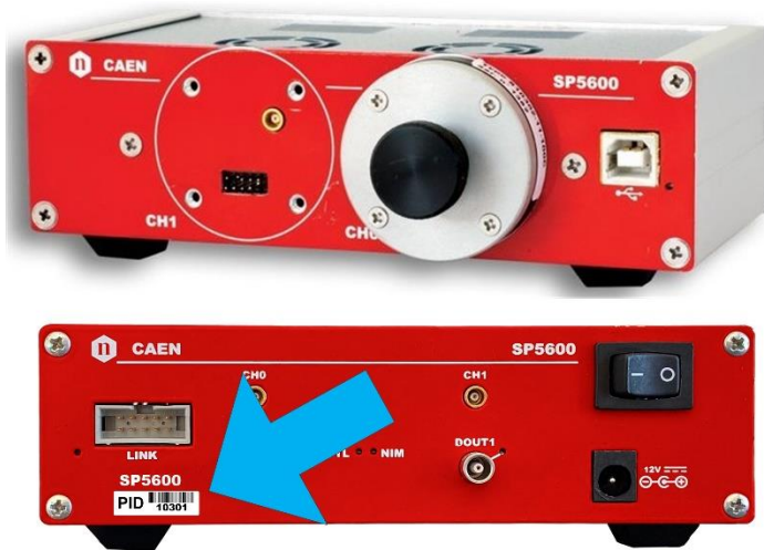
Fig. 3.3: SP5600 - Power Supply and Amplification Unit: PID position is located on the back panel of the module hosting the power input. Same location is adopted for DT5720A - Desktop Digitizer also.
