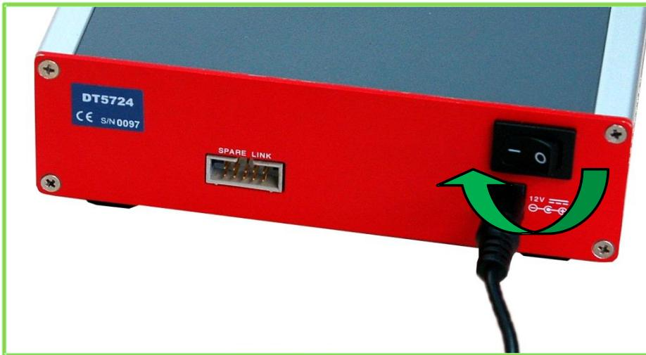
At power on, the Digitizer loads the firmware on the FPGA clearing the output buffer and setting the registers to their default configuration. At the end of the procedure, if succeeded, only the NIM and PLL LOCK LEDs have to stay on.
