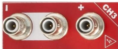
This section is provided with one connector for the positive output and two "bridged" for the negative one, thus allowing to stack two or more adjacent channels. Output ratings: max voltage: 1 kV (Floating up to 5 kV); max current: 1 mA; max power: 0.6W
