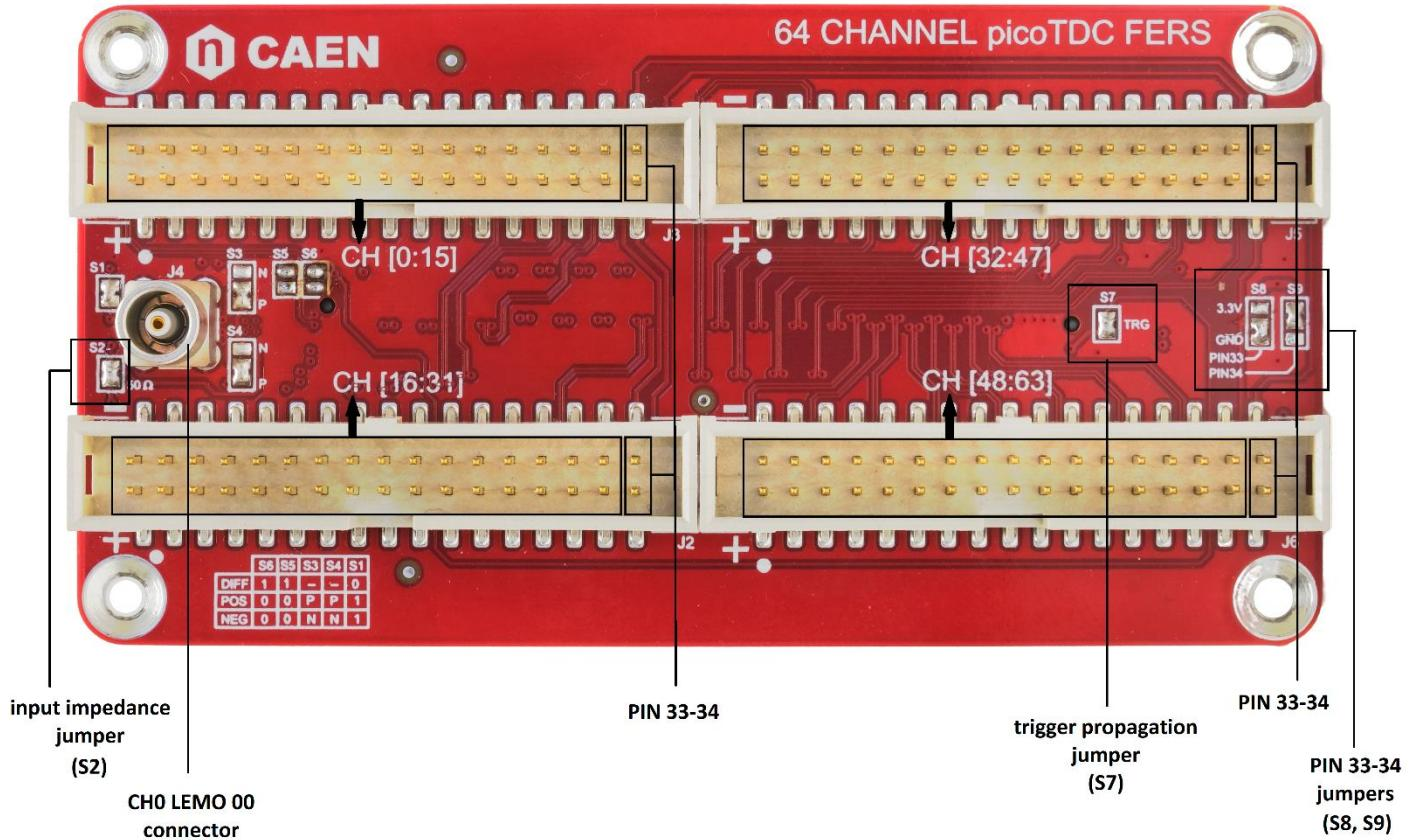
The **LEMO 00 connector**, used to substitute the differential CH0 pin couple, can be enabled/disabled and configured following the scheme in the figure below:
