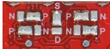
In case of double threshold configuration, the couple of jumpers under each channel are used for one discriminator. Two adjacent jumper couples must then be soldered to set the two thresholds polarity.
