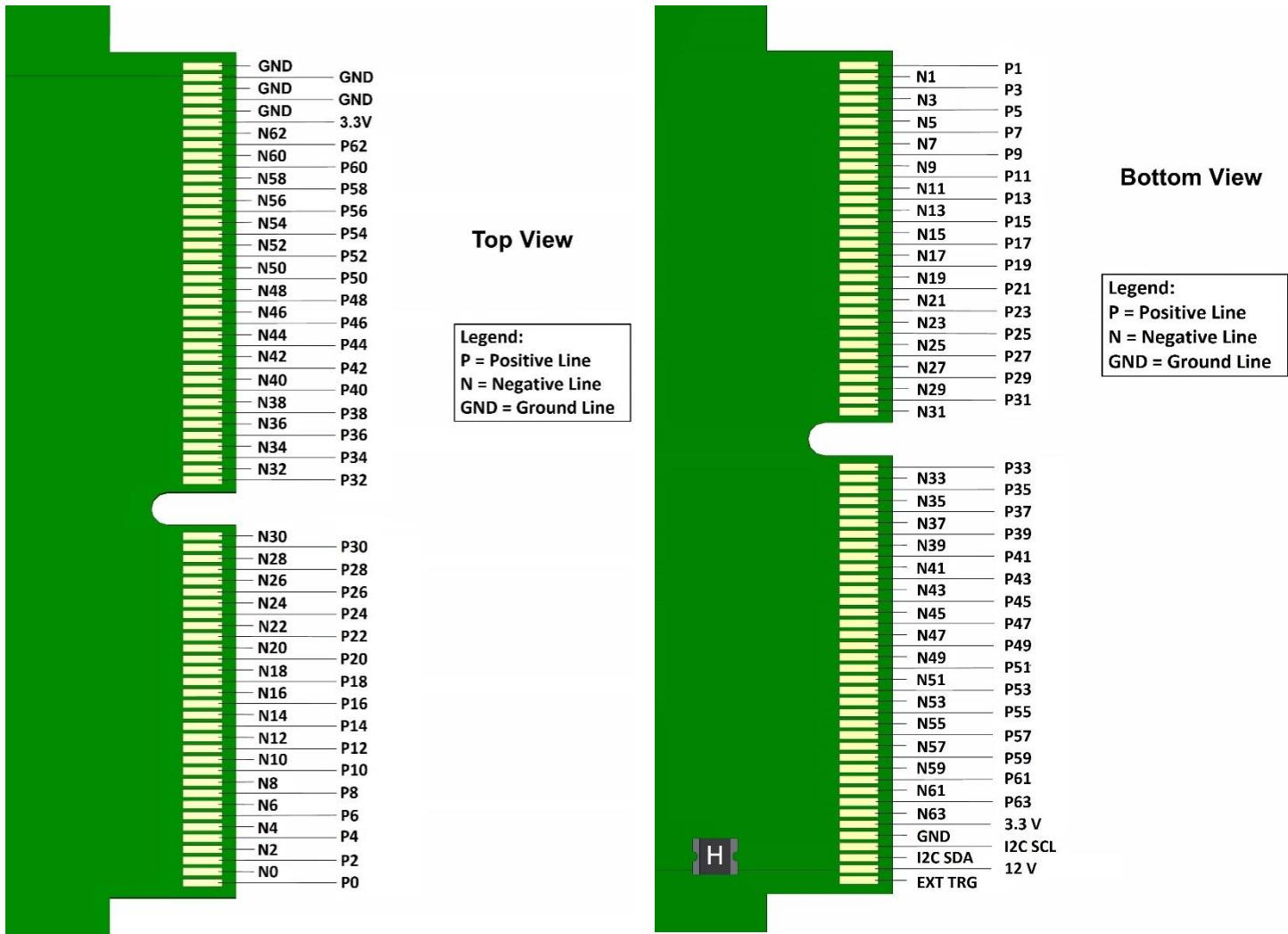
Apart from the differential lines (P-positive and N-negative), the ground lines and the 3.3 V and 12 V lines, three more connections are present:
