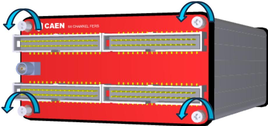
2. Remove the header adapter by taking care of not removing the dark plastic frame around the rear panel. If by chance the frame is removed by the user, it must be reassembled in the direction so that it is externally flush with the header adapter.
