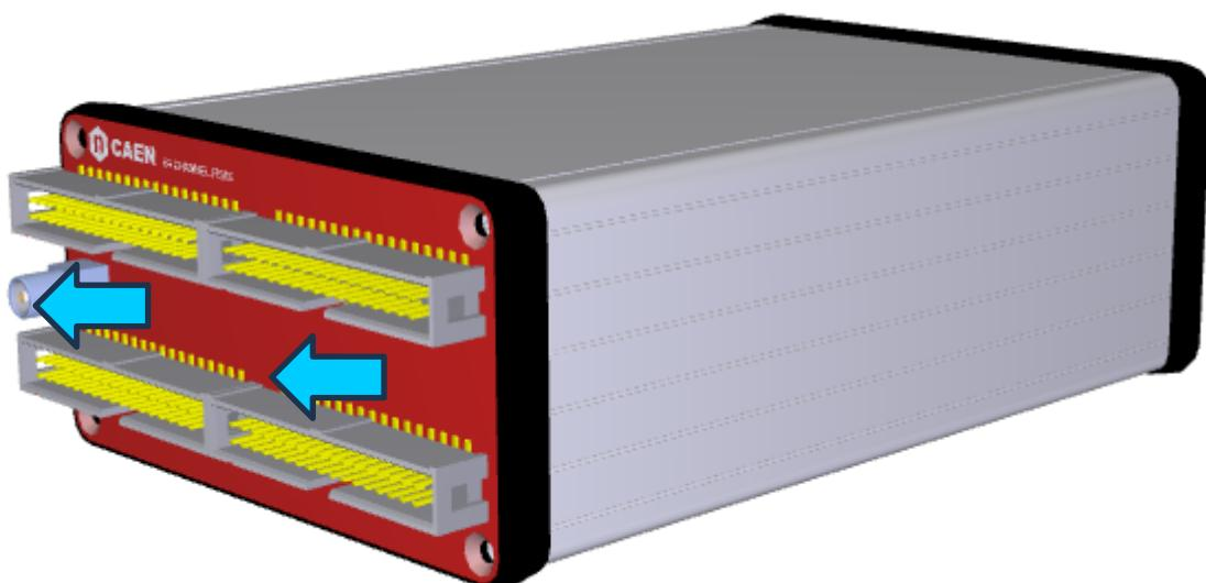
3. Plug the Samtec HSEC8-170-01-S-DV connector of the new header adapter (A5256 in the picture below) into the HSEC8-170 DT5203 edge connector.
