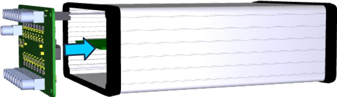
4. Apply again the 4 screws after having checked that the adapter is correctly plugged into the edge connector.
