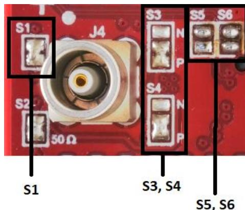
When using the LEMO 00 connector for **ch0** the **input impedance** is set to  $50\ \Omega$  by default. If the user needs a high input impedance ( $\sim 1M\Omega$ ), the S2 jumper should be unsoldered.
