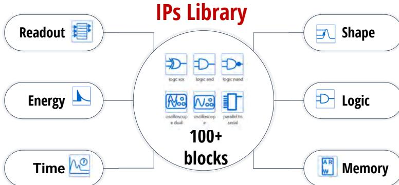
Sci-Compiler is capable of automatically generating VHDL firmware code that implements the functions specified in the block diagram.
