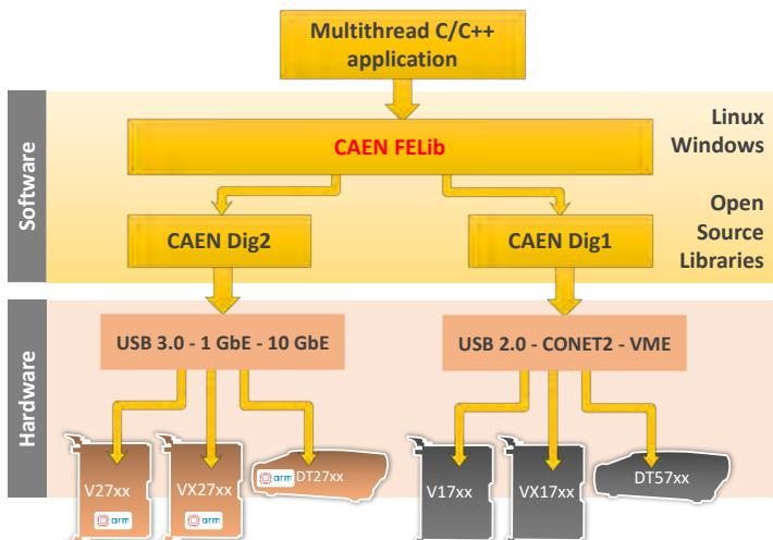
CAEN Waveform digitizers x27xx introduce a new way of accessing the firmware parameters, providing an abstraction of the registers in the form of library parameters that are much easier to understand and use.
