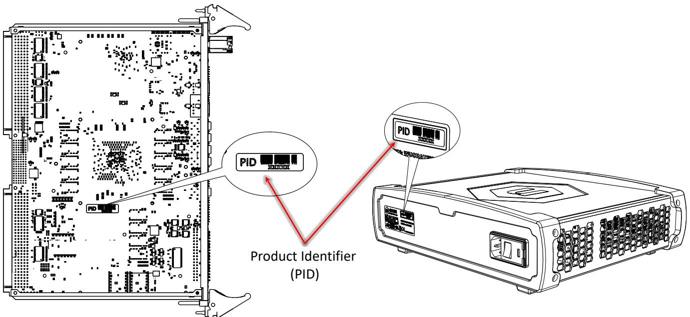
**PID (Product Identifier)** is a unique incremental number greater than 10000 assigned to each CAEN product. It can be found on a label attached to the product (refer to the figure) and is also stored in an onboard non-volatile memory that can be read via the Web Interface.
