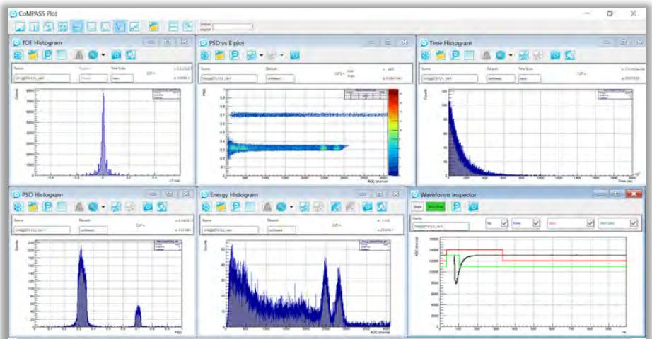
CAEN Multi-PArameter Spectroscopy Software (**CoMPASS**) is the DAQ software for both Digitizer Series 1.0 and 2.0 running the DPP firmware provided by CAEN. It implements a Multiparametric Data Acquisition for Physics Applications: the detectors can be connected directly to the digitizers/MCAs inputs and the software acquires energy, timing, and PSD spectra at the same time.
