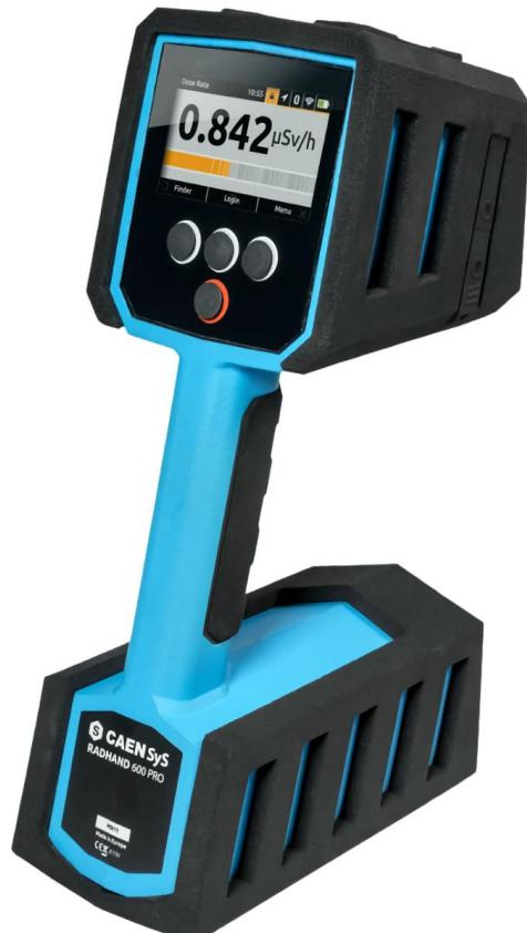
Being part of the CAENSYS DigiWASTE platform, the device can insert measured data and sample information into a central database and, at the same time, write the main information in the memory of selected rad tolerant RFID tags that are part the CAENSYS **RadRFID** family.
