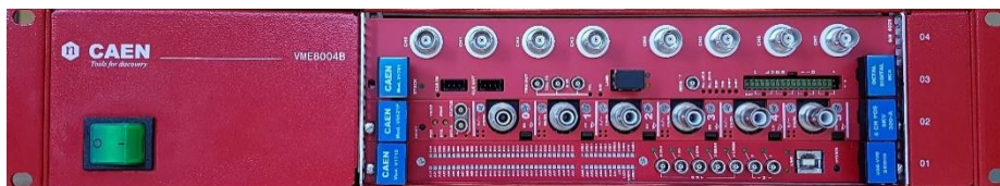
Figure 4: DAQ setup during the measurement with Clovers and Segmented HPGe detectors.
