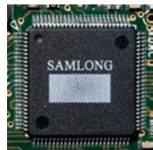
x743 is based on the SAMLONG chip, a Switched Capacitor Array IC. This technology relies on a set of capacitors that continuously sample the analog input signals at a fixed time interval corresponding to the sampling period.
