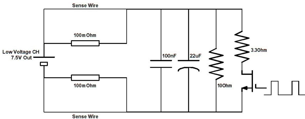
The load is connected to the LV channel, through a couple of cables, whose impedance is estimated 100 mOhm each. The voltage on the load is set to 7.5V, thanks to the sense wires.
