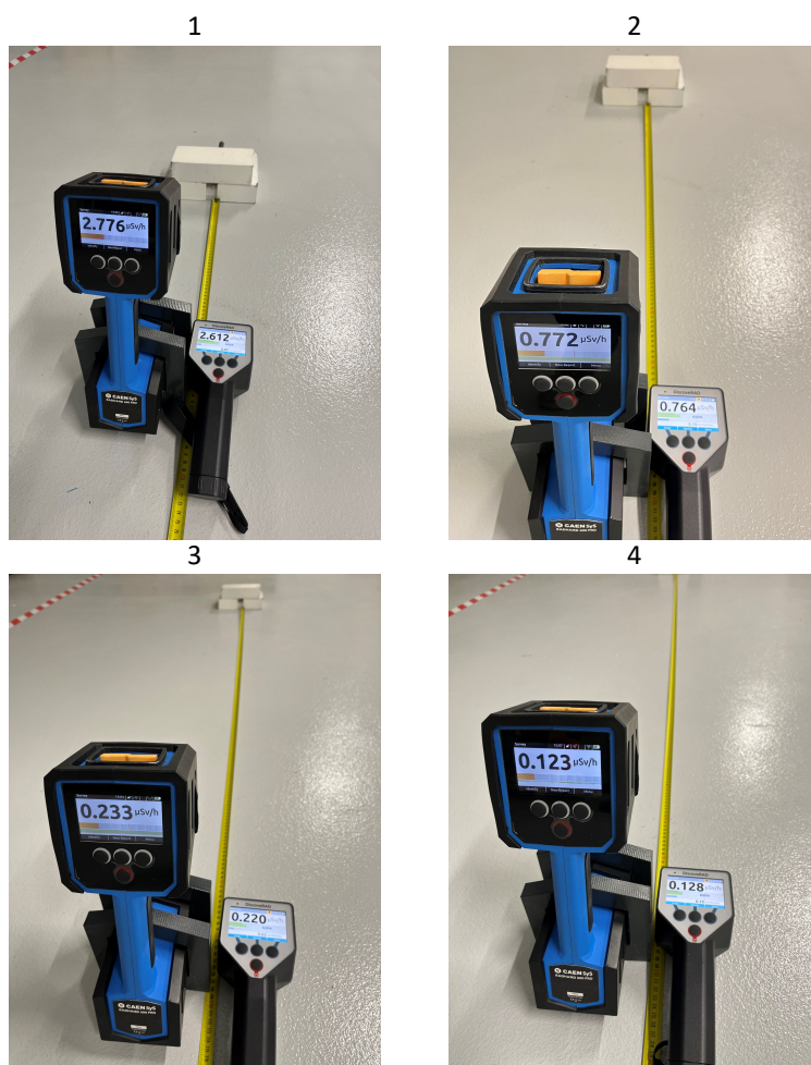
Fig. 4: RadHAND and DiscoverRAD measuring a ^{137}\text{Cs} source with 8.91 \cdot 10^6 Bq of activity at (1) 50 cm, (2) 100 cm, (3) 200 cm, and (4) 300 cm.
