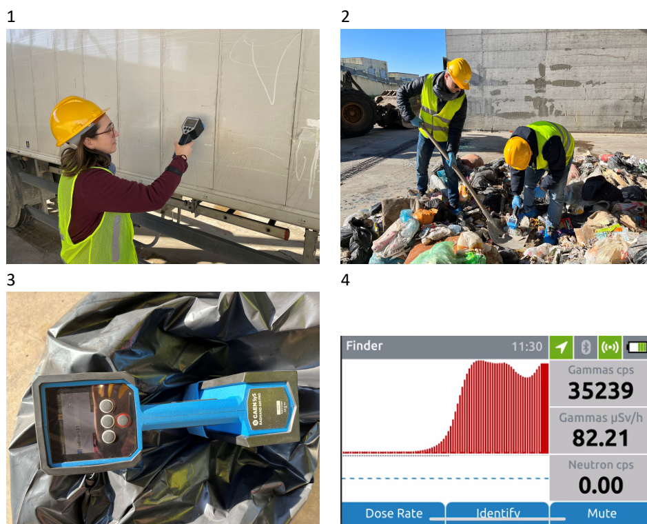
Fig. 1: (1) Localization on the truck wall of the radioactive source; (2) Localization of the radioactive waste among the non-radioactive one; (3) Identification of the radiological source type with RadHAND; (4) Increase of count rate recorded by DiscoverRAD when put close to the source.
