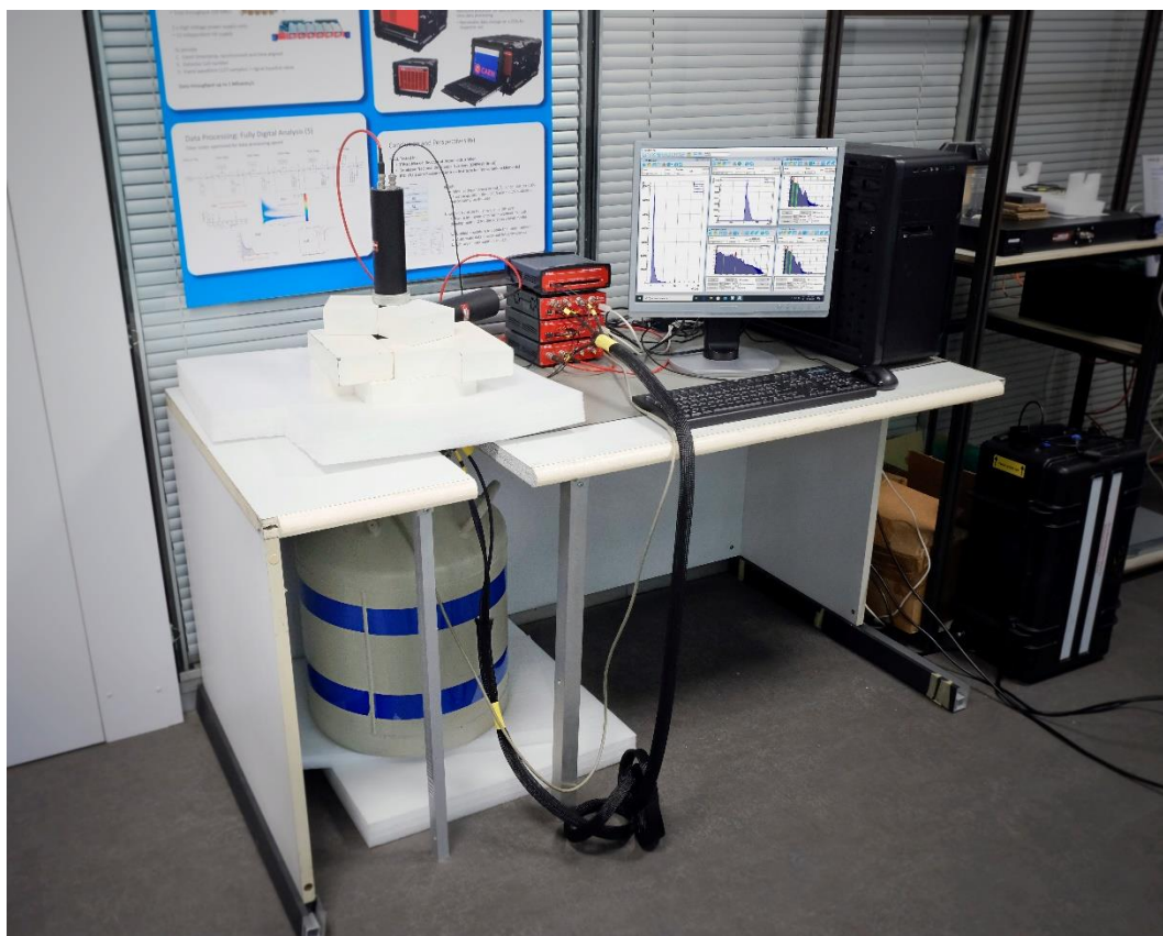
Figure 1: Overview of the PALS demonstrative experimental setup in the CAEN laboratories.
