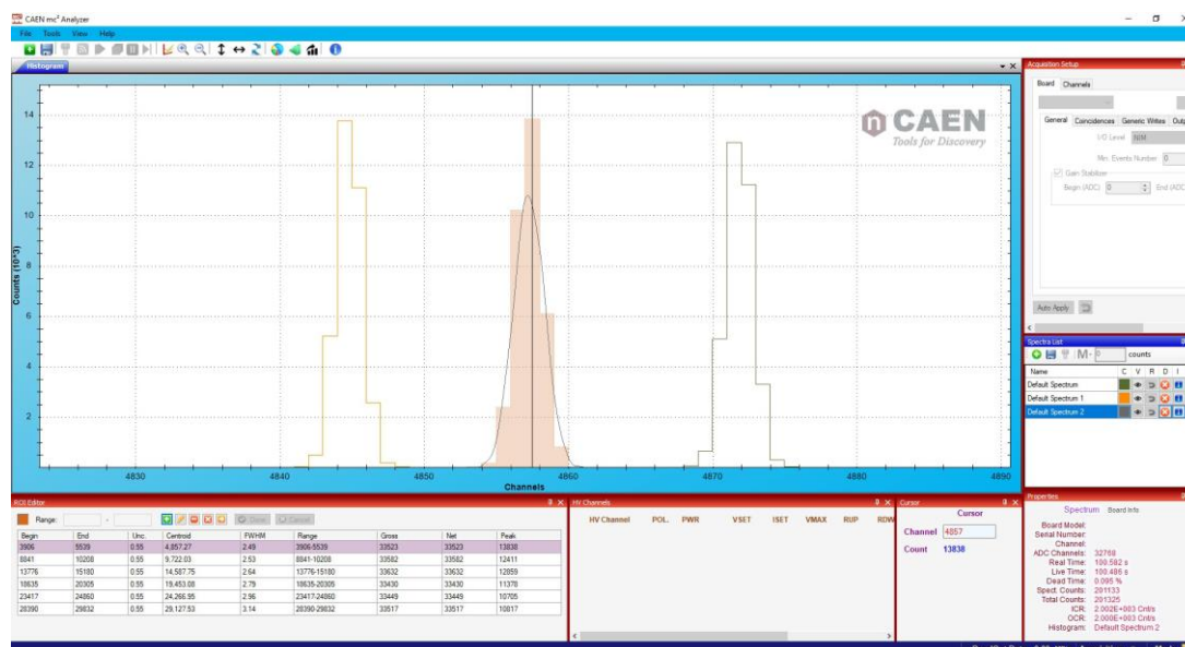
Figure 5: 150mV amplitude peak at gain x1. On the left the peak acquired at 0°C, on the right the peak acquired at 50°C, in the middle the peak acquired at 25°C.
