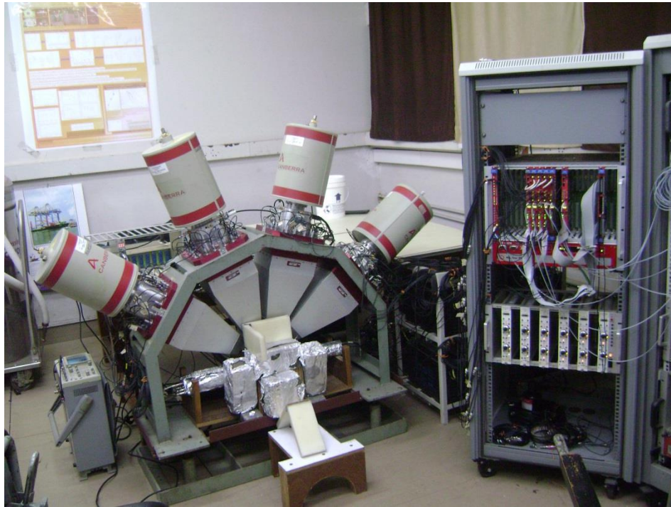
Figure 12: Clover + LaBr 3 experimental setup configuration at the BARC test laboratory.
